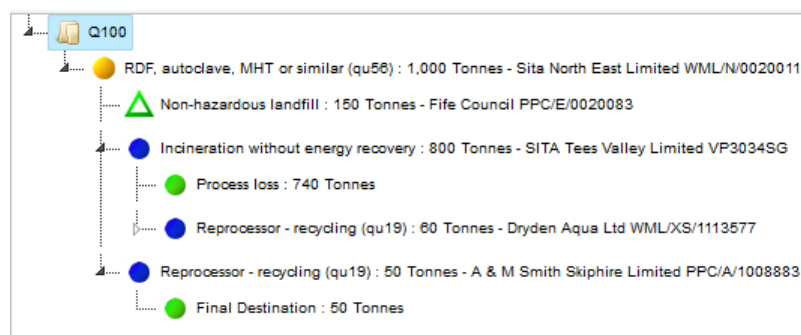
Figure 23. Depiction of residual waste sent to an RDF plant for sorting high calorific waste prior to incineration
